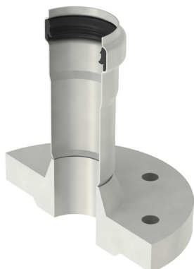
AP connector with socket and flange | acc. to EN 1124 form M1. PN-6 DIN 2631, PN - 10 DIN 2632. PN - 16-DIN 2633
